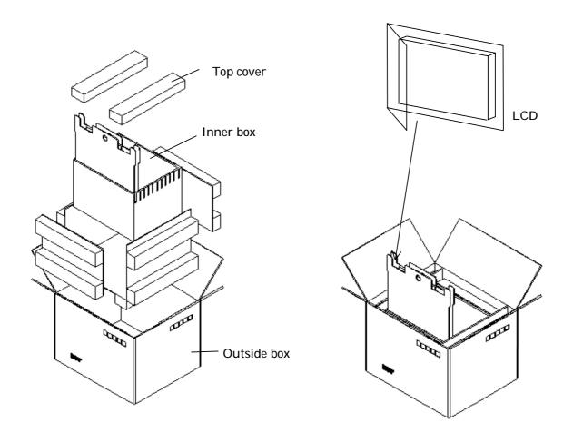
Fig. 1. Illustration of packaging box structure
