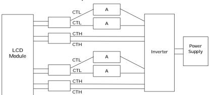
\*3) Lamp frequency of inverter may produce interference with horizontal synchronous frequency, and this may cause horizontal beat on the display. Therefore, please adjust lamp frequency, and keep inverter as far from module as possible or use electronic shielding between inverter and module to avoid the interference.
