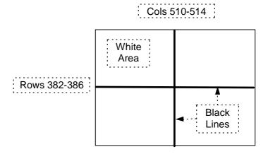
TEST PATTERN FOR IMAGE STICKING TEST
