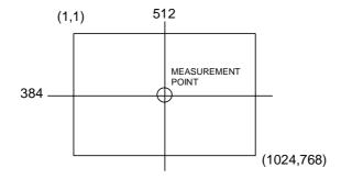
These items are measured when lamp units are assembled into AA150XN02, XN03 or XN04, and using CS1000(MINOLTA) for color coordinates, and CS1000 or BM-5A(TOPCON) for Luminance under the dark room condition (no ambient light) after more than 30 minutes from turning on the lamp unless noted.
